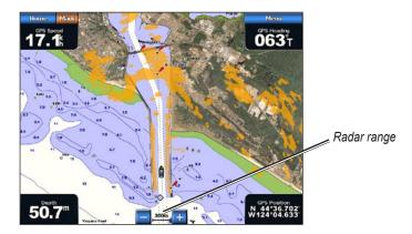
From the Home screen select **Radar** > **Radar Overlay**. The radar picture appears in orange and overlays the Navigation chart. Use the **RANGE** (+/-) keys (GPSMAP 4000 series) or the same leaves (GPSMAP 5000 series) to zoom in and out. Zooming while panning the map only affects the zoom scale of the map. The radar range remains the same. Zooming while the map is locked on the boat (not panning) affects the zoom scale of the map and the radar range.
